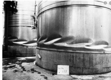
*Buckled axially compressed axially stiffened cylindrical shell.*
