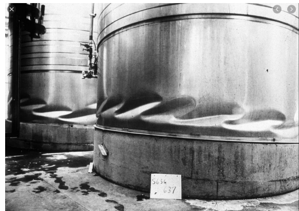
Buckled axially compressed axially stiffened cylindrical shell.
