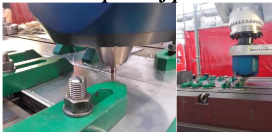
Friction Stir Welding, on ABB IRB 8700 robot
