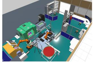
advance industrialization performance. as you can see in the opposite illustration, the workshop is made up of kuka robots and several numerically controlled machine tools, as for the IoT layer is made up of different sensors and smart cameras. In addition, the controlling of the various operations is carried out by wonderware numerical platform.
