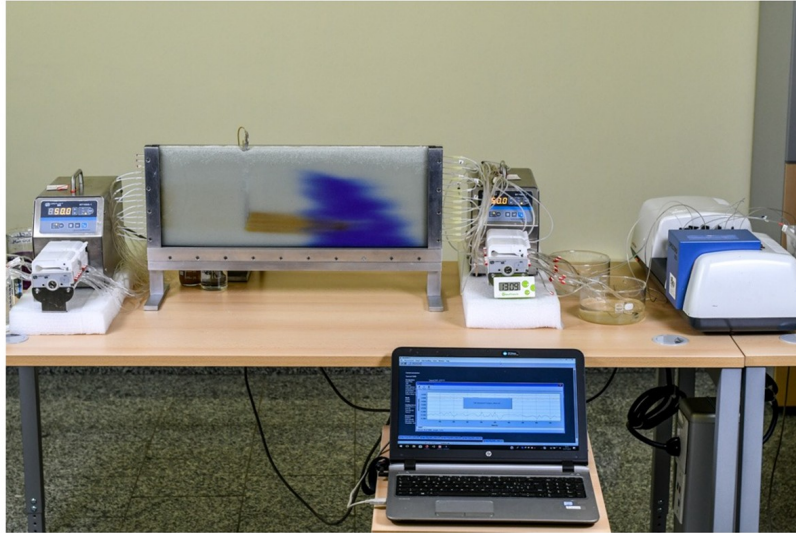
Figure 4 Experimental setup for the simulation of emulsified zerovalent iron injection and propagation in 2D vertical geometry (Groundwater Engineering Group – Politecnico di Torino )
