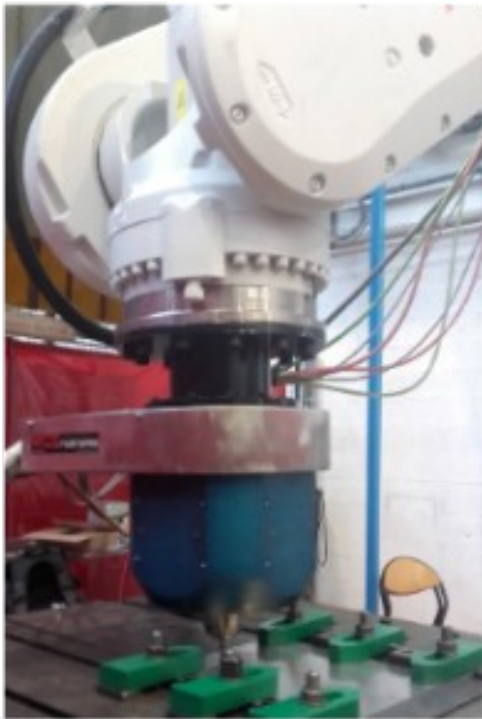
Friction Stir Welding on ABB IRB 8700 robot
